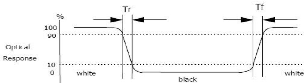
Response time is the time required for the display to transition from white to black (Rising time,  $T_r$ ) and from black to white (Falling time,  $T_f$ ) for additional information.
