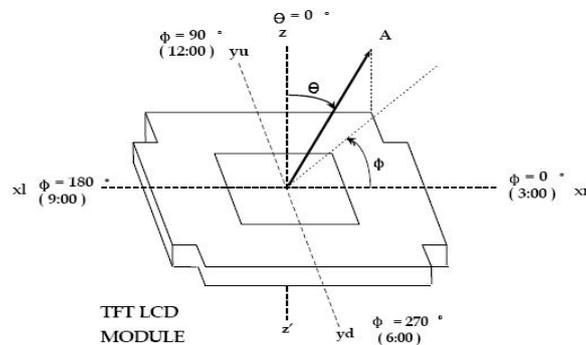
Viewing angle is the angle at which the contrast ratio is greater than 10. The angles are determined for the horizontal or x axis and the vertical or y axis with respect to the z axis which is normal to the LCD surface.
