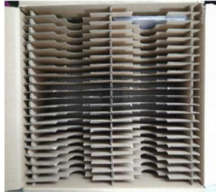
Take 2 bags of product to place into the carton, make sure they are surface to surface. Put a piece of EPE pad between the carton and the separator to protect the products.
