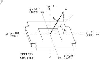
Viewing angle is the angle at which the contrast ratio is greater than 10. The angles are determined for the horizontal or x axis and the vertical or y axis with respect to the z axis which is normal to the LCD surface.
