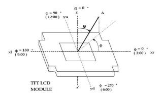
Viewing angle is the angle at which the contrast ratio is greater than 10. The angles are determined for the horizontal or x axis and the vertical or y axis with respect to the z axis which is normal to the LCD surface.
